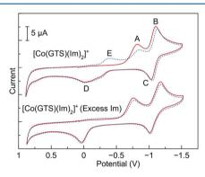
**Figure 4.** Cyclic voltammogram of  $[Co(GTS)(Im)_2]^+$  before (top) and after (bottom) addition of excess imidazole. The first scan is shown as a solid red line, while the second scan is represented by small blue dashes. This experiment was performed at 25 °C in DMF solution with 0.10 M TBAP electrolyte at a scan rate of 100 mV/s. The potential is referenced to SCE on the basis of the position of the Fc/Fc<sup>+</sup> couple as an internal standard.
